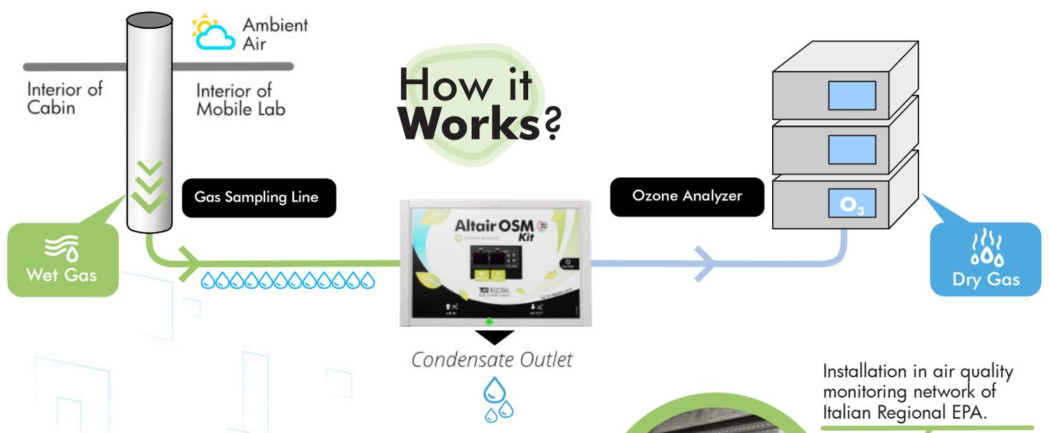
It is well known that errors in measurement occur in some period during the year due to condensation into the sampling tube of analyzer.
