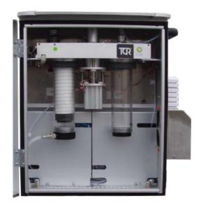
A high reliability OPC (optical particle counter) for real time monitoring of PM10, PM2.5 and PM1 is available as an option. With this device is possible to monitor in real time the particulate quantity during sampling and to approximately know in advance what will be be the result of the particle load in the filter membrane. The analyzer also measure the particles size distribution (24 classes within the range 0,35-40  $\mu$ m)
