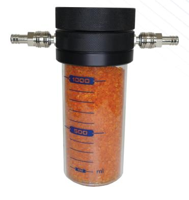
X-TRAP is also used in the sampling of moisture in gasses emitted by industrial processes as prescribed by EN 14790. The silica gel is introduced in the container, and this is first weighted. After sampling, the container is weighted again and by difference the accumulated moisture content is obtained.
