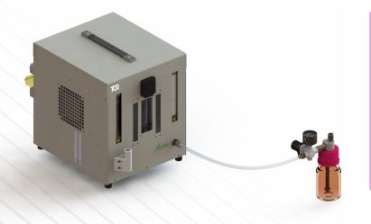
DDS AERO is also zero air generator, it can filter particles with Hepa filters up to 99.999 % and can have a line with silica gel dryer, purafilter with activated carbon mixed inside for pollutant abatement and air purification.
