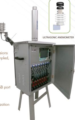
The **ECHO TUBE** sampler has been studied and designed for sequential sampling on vials for gaseous compounds at flowrate from 100 to 2000 cc/min, and to comply to regulation request on sampling field, prescribed in the EN 14662-2:2005 "Ambient air quality – Standard method for measurement of benzene concentrations – Part 2: Pumped sampling followed by solvent desorption and gas chromatography".
