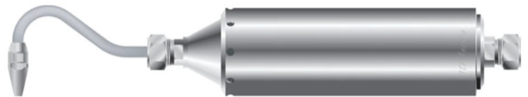
Fig.2 Assembled Impactor with nozzle for sampling in horizontal position
