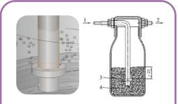
Single Nozzle Version Particles: range 0.5 - 5  $\mu$ m Aerosol concentration: >10<sup>7</sup> p/cm<sup>3</sup> Flow: 1 - 100 l/min Pressure: 0.1 - 4 bar
