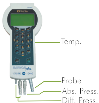
Connection to pressure and temperature sensors
