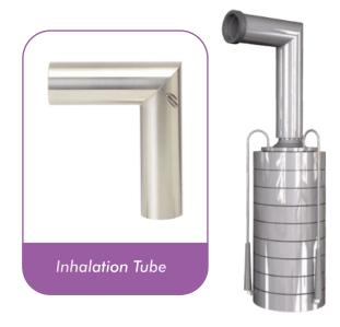
By analyzing the drug deposited on the individual stages and the final filter, the Fine Particle Fraction, the Fine Particle Dose, the Mass Median Aerodynamic Diameter (MMAD) can all be calculated.
