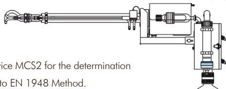
Condensing and adsorbing device MCS2 for the determination of PCDD/PCDF in compliance to EN 1948 Method.
